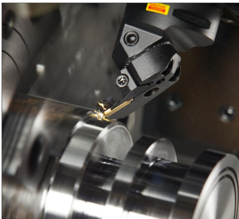
Figure 10 . Tungsten carbide cutting tool.
