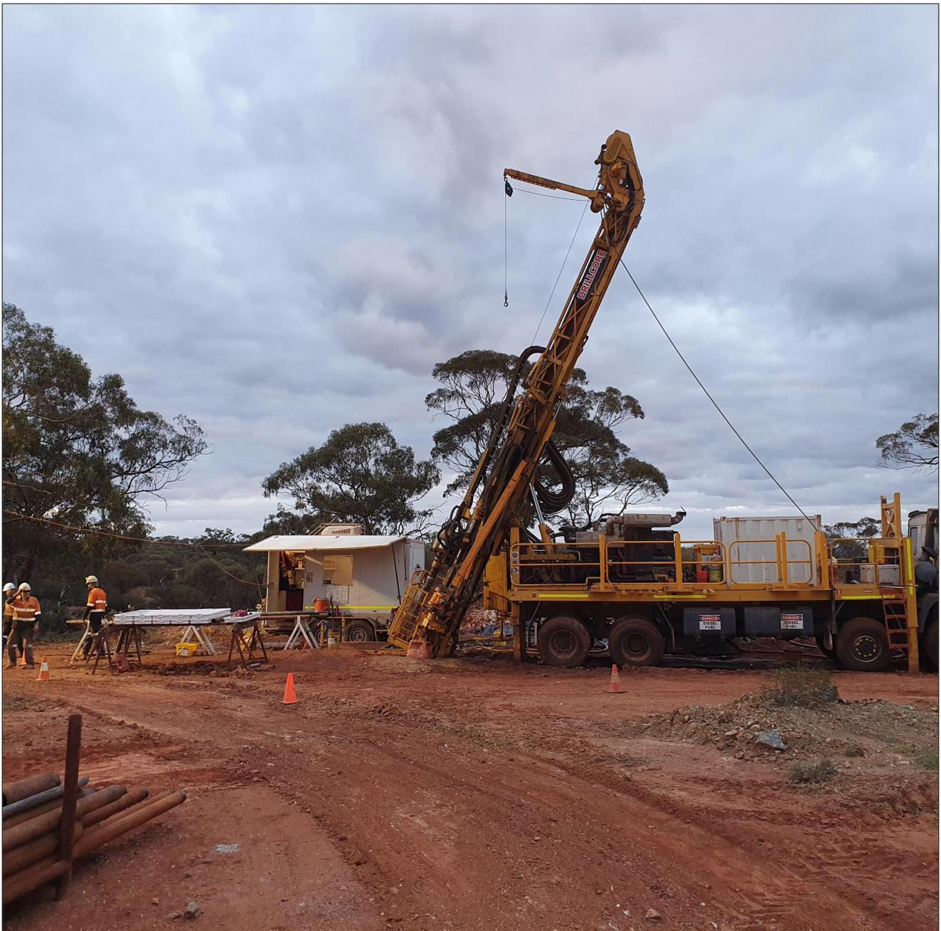
Figure 2. PQ metallurgical drilling underway at Mt Mulgine
