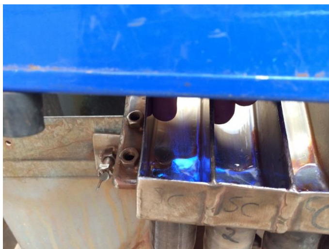
Figure 9 – Wet table (Kilba) Concentrate highlighting Scheelite under UV
