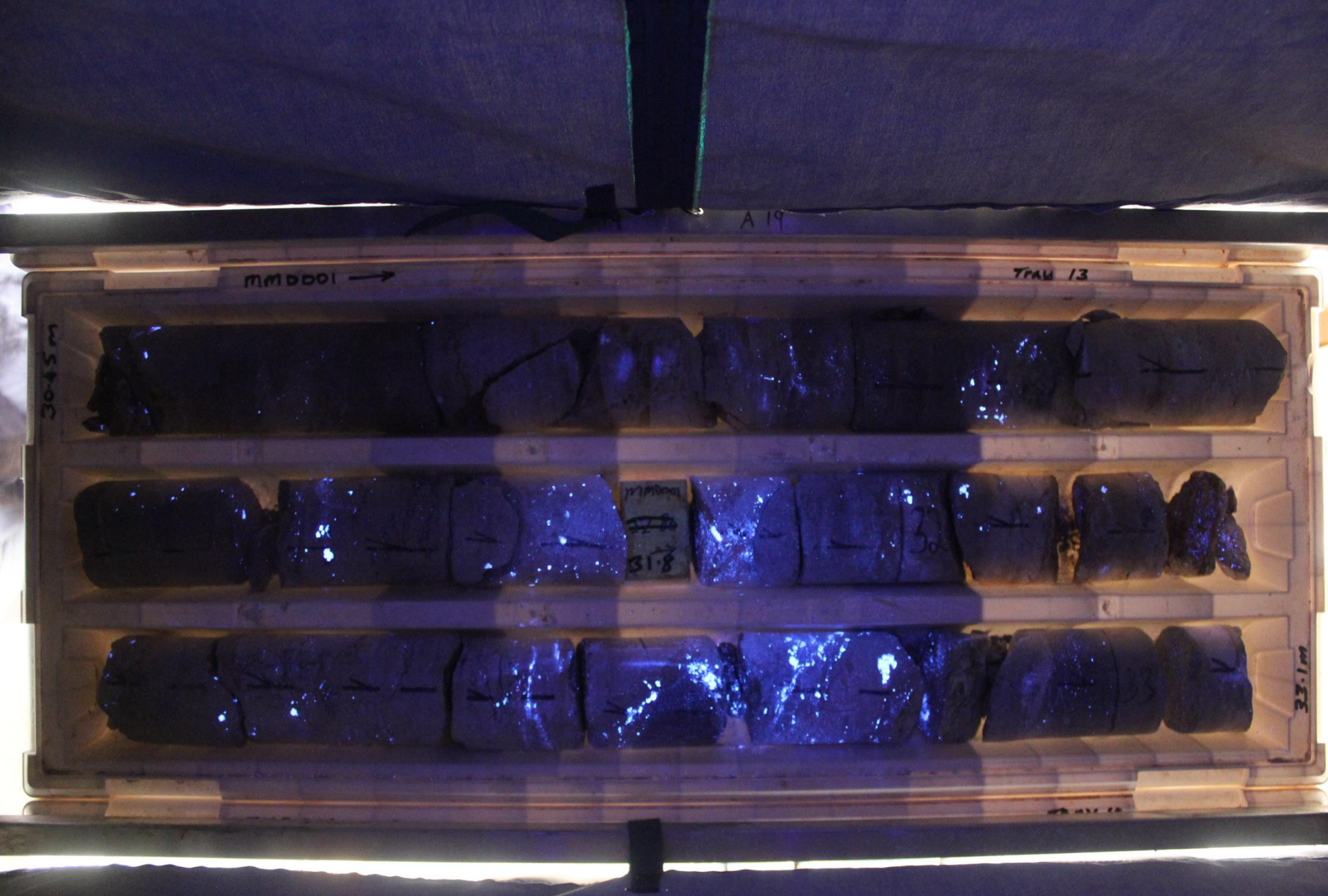
Mulgine Hill Drill Core Sample Showing Coarse Grain Scheelite (UV light)
