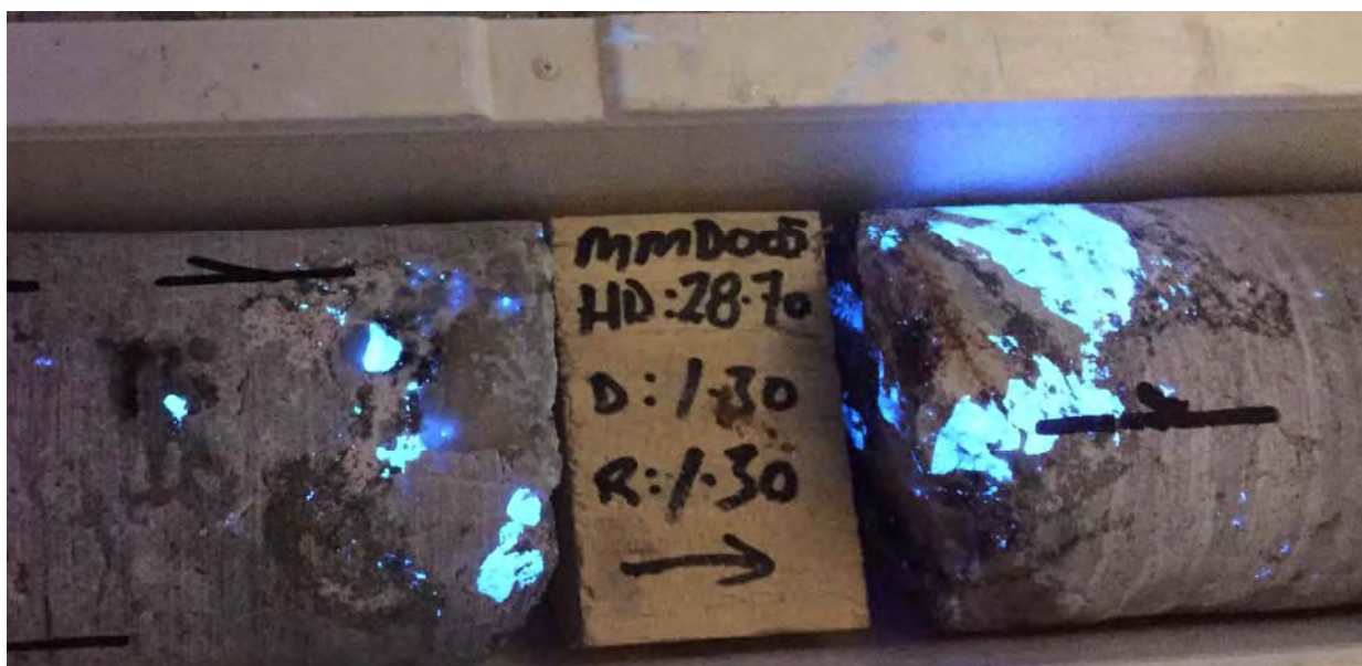
Figure 6: Diamond core from August 2016 drilling program showing coarse grained scheelite under UV
