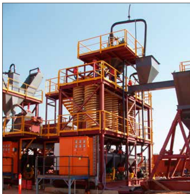
Figure 5: Bank of spirals in modular processing plant (in-situ prior to dismantling and relocation).
