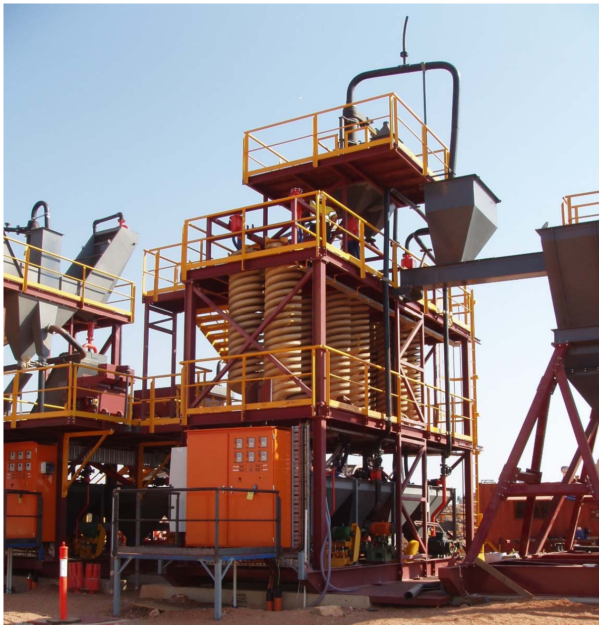
Figure 5: Bank of spirals in modular processing plant (in-situ prior to dismantling and relocation)
