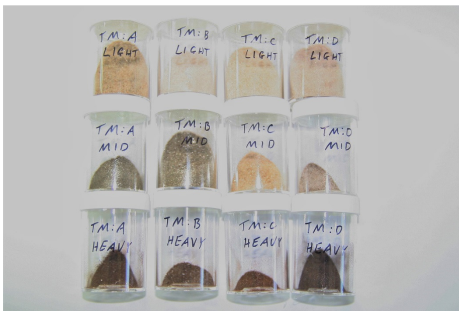
Figure 5 – products from heavy liquid test work showing the separation of “heavy” minerals containing greater than 75% of the tungsten bearing minerals.
