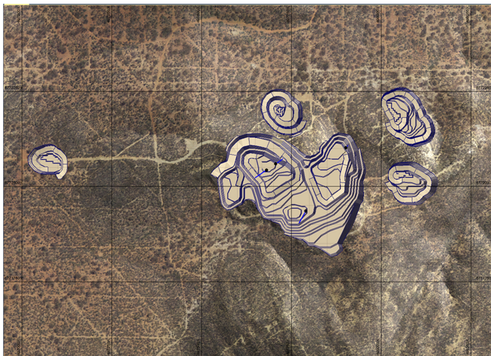
Figure 6 – Plan showing new pit designs and location of geotechnical diamond drill holes.
