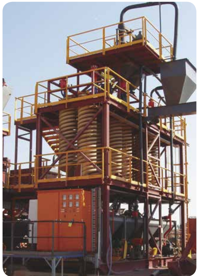
Figure 4 - Bank of spirals in modular processing plant (in-situ prior to dismantling and relocation)
