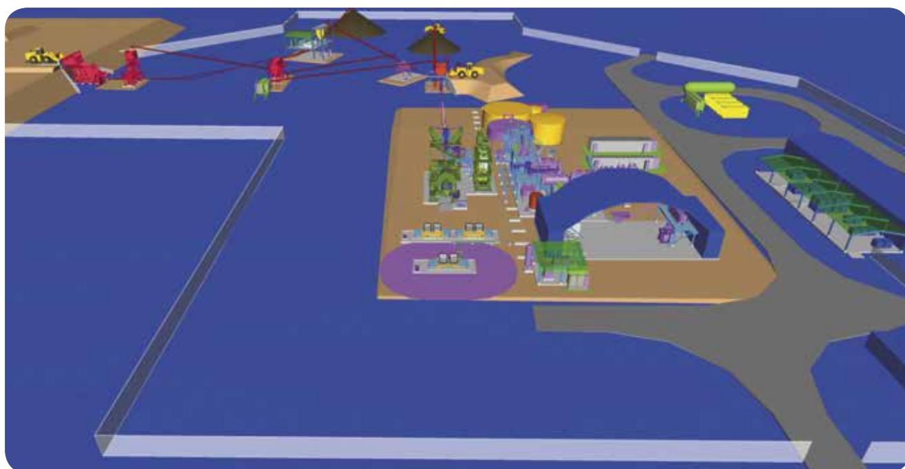
Figure 8 – View of processing plant incorporating crushing, screening and x-ray ore sorting, gravity, flotation and final concentrate preparation.
