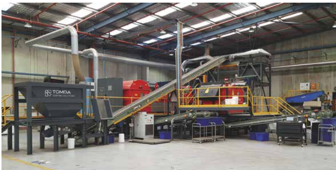
Figure 11 – X-ray ore sorting trial at Tomra facility in NSW
