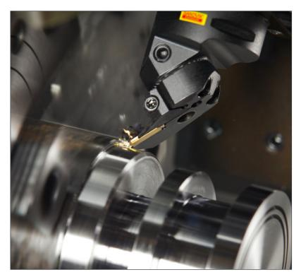
Figure 10 . Tungsten carbide cutting tool.
