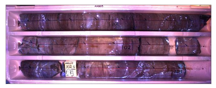
Figure 3. UV Photograph of typical mineralised core in MMD015 from 100.5m to 103.0m recovered from the current Mulgine Trench drilling program, showing coarse grained scheelite associated with quartz veining. The corresponding zone in the twin hole MMC319 assayed 4m at 0.11% WO3 from 100m, within an overall mineralised envelope of 108m at 0.11% WO3, 70 ppm Mo from surface.
